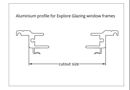
The Land Rover Defender Pick-up sliding window with the original Land Rover dimensions 905 mm  $\times$  365 mm with 4  $\times$  radius 70 mm. This type of window can also be mounted in a Land Rover Defender 110 hard top.
